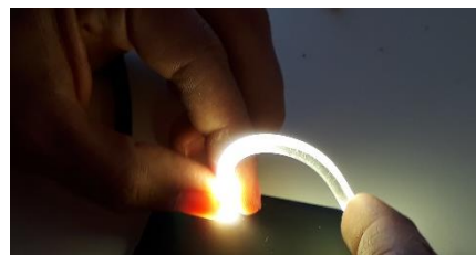
After proper sanding, one side of the fiber cable glows when bent, due to the escape of light.
