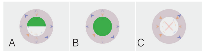
Figure 2: Feedback mechanism in the Central Circle design. A. Half activation B. Full activation. C. Incorrectly performed bend gesture.
