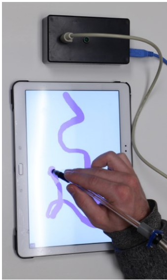
Figure 1: The FlexStylus system, demonstrating a mapping of absolute bend to line weight.
