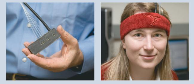
Figure 1. The arrangement of detectors and light sources on an optical probe used for functional near-infrared spectroscopy can differ depending on the probe's design. This probe has five light sources and one optical detector.
