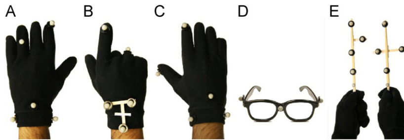
Fig. 7. Marker arrangements: left glove (A), right glove, squeezing (B), right glove for unimanual multipoint and trigger (C), glasses (D), left laser pointer (E), right laser pointer (F).
