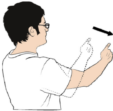
Fig. 4. Remote selection technique—Breach gesture. The dotted lines indicate the initial state (close to the body), and the plain lines indicate the selection state (passed the invisible threshold).
