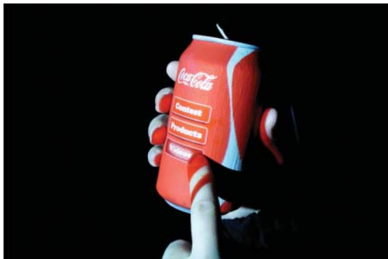
Figure 1. The DynaCan is a pop-can computer that embodies a cylindrical interactive display and demonstrates an application in mass consumerism.
