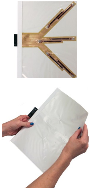
Figure 3. Left: the bend sensors layout at the back of the prototype. Right: the prototype used in the study.
