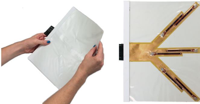
Figure 3. Left: the prototype used in the study. Right: the bend sensors layout at the back of the prototype.
