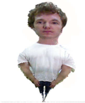
Figure 3. Textured 3D model with hemispherical distortion. When reflected off the convex mirror onto the cylinder, this produces a 3D model with proper proportions.
