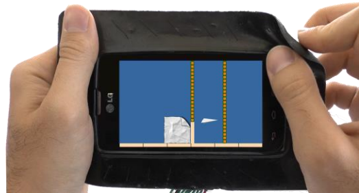
Figure 1. The player bends the flexible case to shoot paper airplanes to break the wall in the PaperNinja game.
