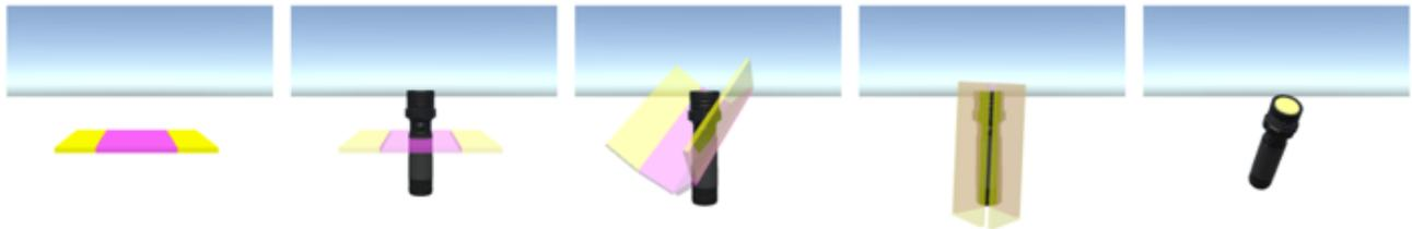
Figure 3. Example of HaptoBend mapping process to a virtual object: the virtual object appears (left); the participant determines their preferred shape (middle images), before notifying the experimenter that the shape is ready; the virtual model of HaptoBend disappears and the participant controls the rotation of the virtual object with the prototype (right).
