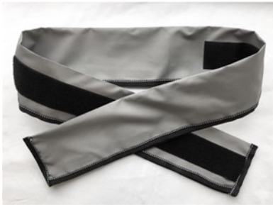
Figure 2: SensArt cover contains the belt and all electronic components
