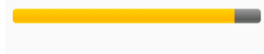
Figure 6. Example control using the angle calculated between the x- and y-values. The -180-180 range is mapped to a linear level control.
