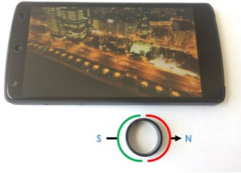
Figure 1. Setup of the prototype. Top: Mobile device (Nexus 5), Bottom: Magnetic ring (diametrically magnetized). The ring can be placed anywhere around the device as long as its movements are within the detection range of the device's magnetometer.
