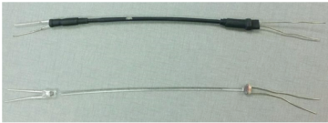
Figure 3. Optical-based bend sensor. (Top) Finished sensor wrapped to prevent light leakage. (Bottom) Internal components: LED, optic fiber, photosensor
