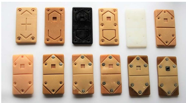
Figure 3. Iterating through prototypes in silicone lets researchers achieve quickly the correct design considerations of form factor, ergonomics and sensing requirements.
