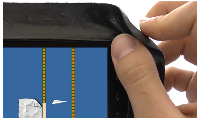
Figure 1. Flexible devices offer deformation as a source of input. In this game, bending the top right corner towards the user fires a paper arrow [6].
