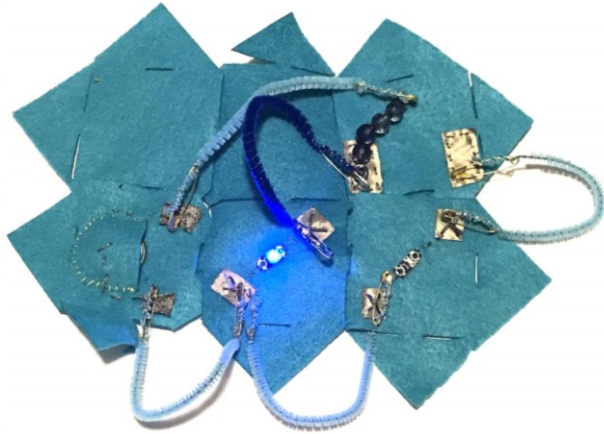
Figure 7—A simple circuit made with the medium-fidelity bits, including a tilt sensor that lights up.
