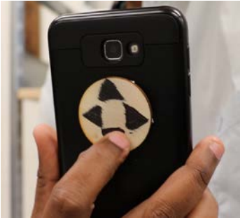
Figure 2. Low-Fidelity touchpad BODI prototype.
