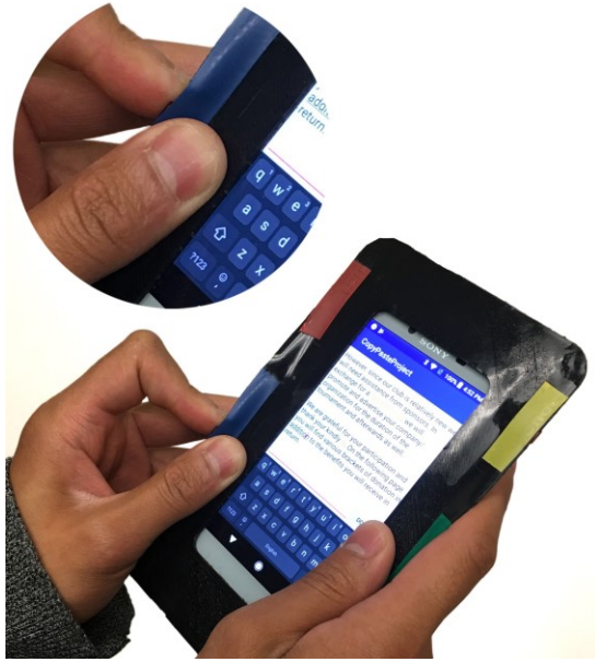
Figure 2: A deformable interactive device, BendAide, that fits around a mobile phone. It uses bend interactions to provide alternative controls during complex tasks like text manipulation.
