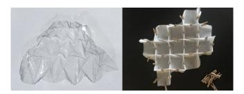
Figure 2: Building the shape-changing swatches (left) the mold, (right) securing the folds with wooden clips
