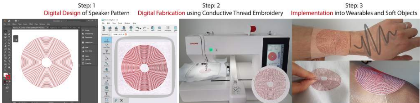
Figure 1: Soft Speakers: digitally embroidered audio and haptic actuators on fabrics in three steps: 1) Digital design of the speaker pattern using Adobe Illustrator or Artistic Digitizer Software, 2) Digital fabrication using conductive thread in a digital embroidery machine; 3) Implementation into soft interfaces and wearables
