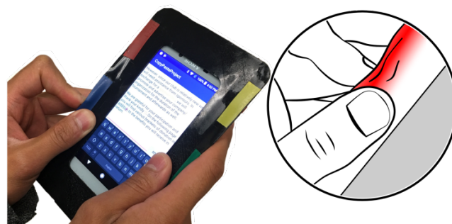
Figure 1: BendAide is a 3D printed case that is fitted around a touchscreen mobile device. Its deformable bezel detects bend input, providing an alternative interaction modality to touch in support of complex text tasks.
