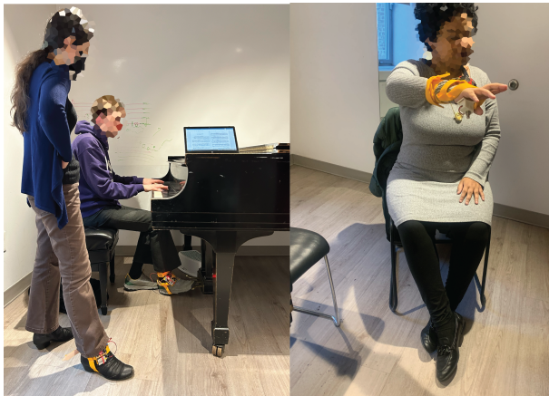
Figure 7: Image on Left: Designed placement of the TapTap in a music lesson scenario, with both T1 and S1 wearing the device on their right feet. The image on Right: S4 experimented with wearing the TapTap on their right arm for improved comfort.
